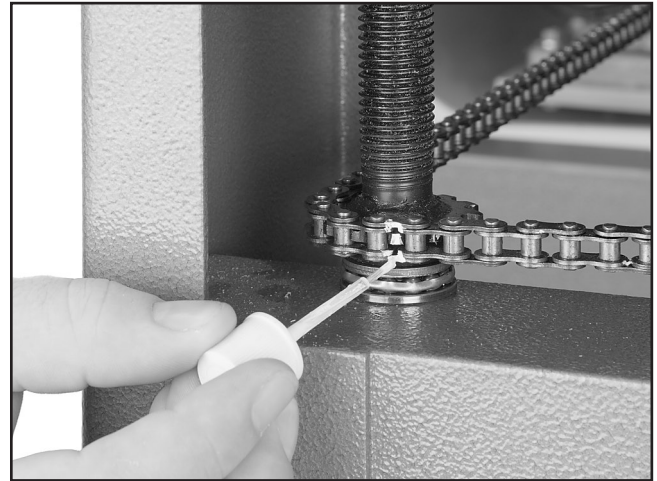
Figure 42. Marking sprocket tooth and chain.
